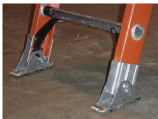
Firm Base Set both feet level and on the pads
