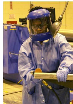
Figure 4.5 Veronica Thomas, a sheet metal mechanic, de-burrs an inconel steel part for installation on the C-130 IRSS. U. S. Air Force photo by Chad Langston.
