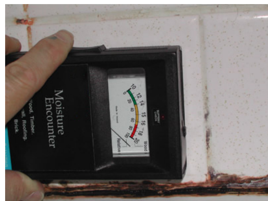
Figure 4: Moisture meter showing damp baseboards
