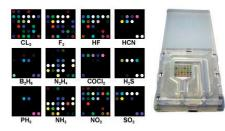
A postage stamp-sized optical sensor array for toxic gases, showing the color changes associated with a few representative poison gases
